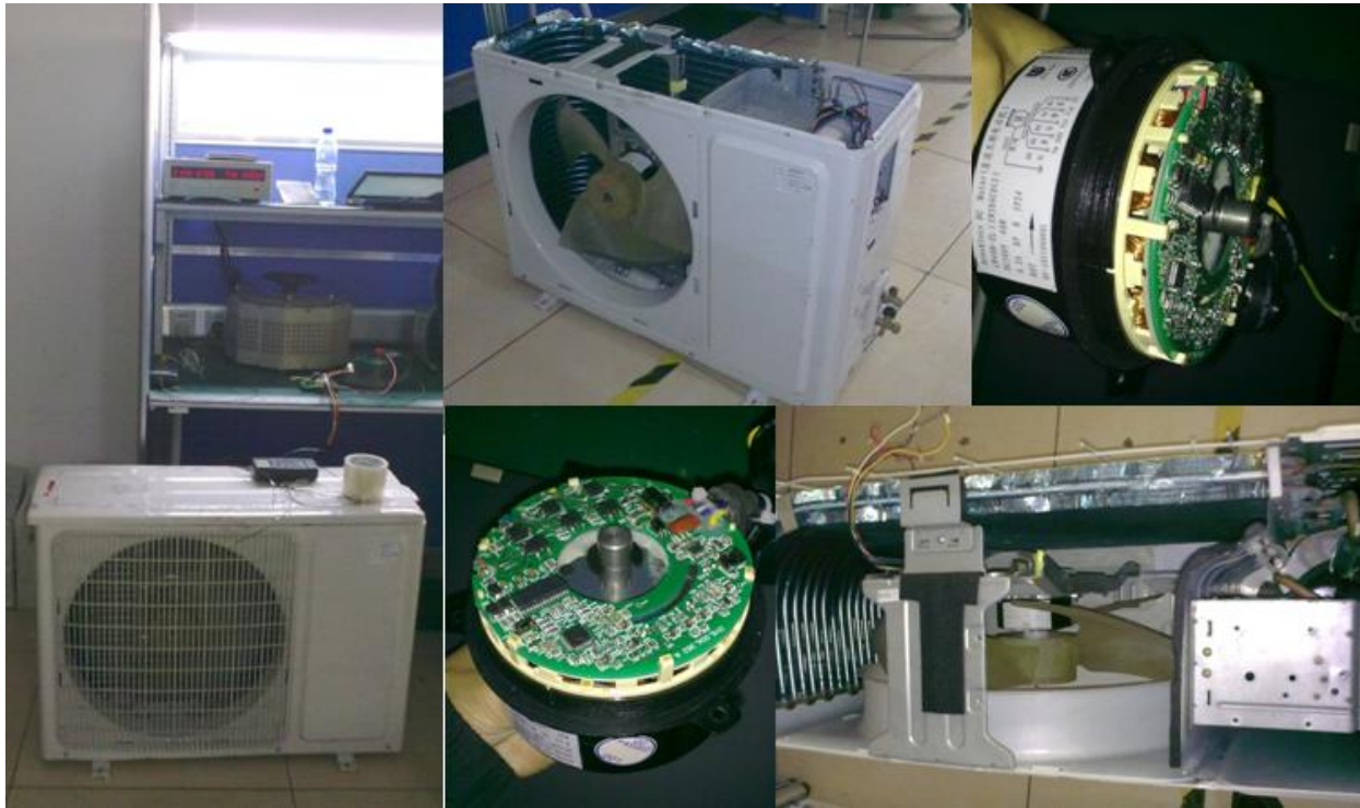
Figure 9: Commercial Air-conditioning split system, showing the motor drive card housed on the back of the BLDC fan motor
